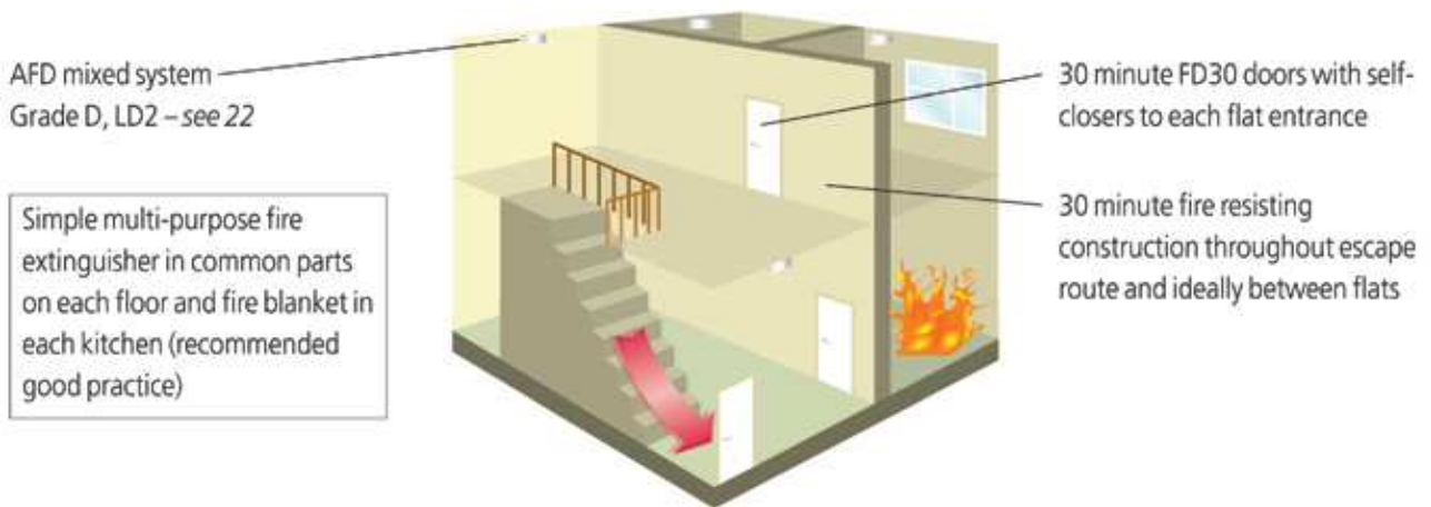
figure D10: two storey building converted to flats
